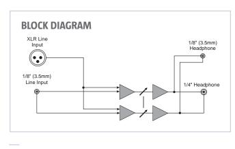
**Cut through the Crowd Noise.** The RemoteAmp is a simple battery-powered personal headphone amplifier. Use the RemoteAmp as an IFB earpiece or headphone amplifier, or as an on-stage monitor headphone amplifier. This low-distortion, ½ watt amplifier will cut through the crowd noise without distortion.
