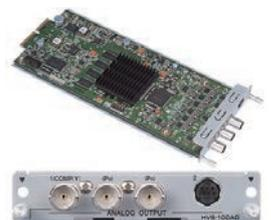
**HVS-100PCI** available for slot A or B**PC (HDMI/VGA) Input Card**
