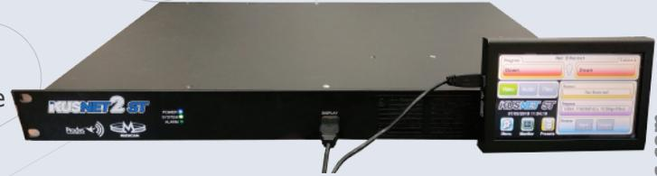
Ikusnet2 ST can be operated either from a detachable touch panel or built-in web interface.
