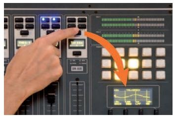
FORUM's configuration allows any signal present within the system to be freely assigned to any control channel, and signal distribution configuration is done on the control surface itself.
