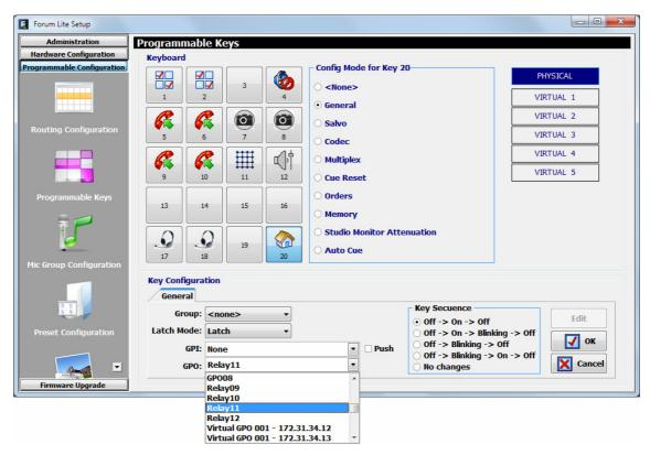
In order to be able to configure the programmable key (or edit a previously created configuration), you have to press the "Edit" button, to active and allows you to configure the following fields:
