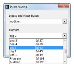
The routing toward MPX internal summing buses is saved on console configuration and it will appear in the "Routing Configuration" submenu when the active configuration is read.
