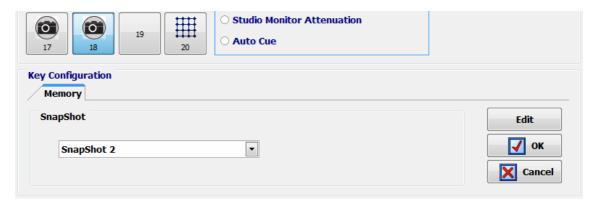
**IMPORTANT NOTE 1:** When you press the key the configuration stored in the selected memory is directly loaded into the console. In this case <u>no confirmation is requested</u> (the system will ask for confirmation only when the memory is loaded from the "MEMORY" menu: see section 3.3 of this manual).
