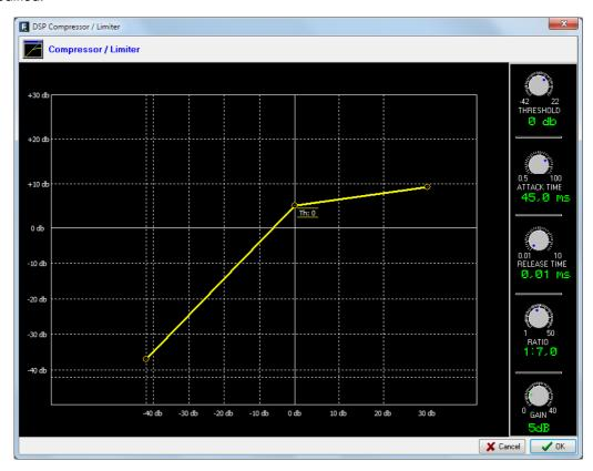
Dynamics processors are used to modify the dynamic ranges of an audio signal to adapt it to specific needs or to produce certain sound effects. A compressor enables you to reduce the dynamic range of the signal. Your purpose may be to adapt a signal with a very broad dynamic range to a circuit that will not support such wide variations in level, or to generate a certain sound in a signal.
