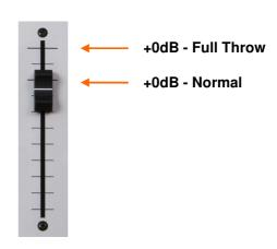
"Digital Nominal Level": allows you to configure the digital nominal level of the console. By default, the nominal level of AEQ consoles for <u>digital signals</u> is -20dBFS. There is an adjustment margin of +/-12dB by means of gains configuration.
