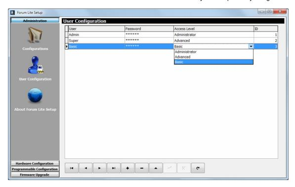
The lower part of the "User Configuration submenu includes a set of standardized buttons to manage the list of registered users:
