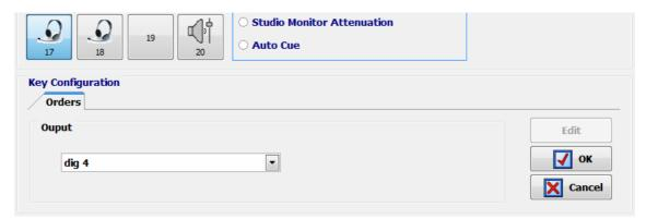
These keys works as follows: when you press and keep pressed the key you send to the selected output the orders microphone (any routing previously defined for that output is deactivated). When you stop pressing the programmable key, you stop sending the orders microphone and the previous routing is recovered.
