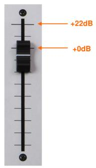
Detail of 100mm fader calibration
