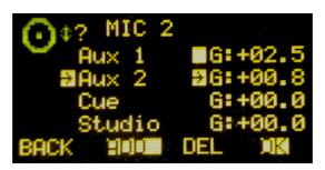
In the example, the send from "MIC 2" input to the summing bus "Aux 1" is linked to the fader (there is no arrow in the cross point) and the send to "Aux 2" is pre-fader (there is an arrow in the cross point).
