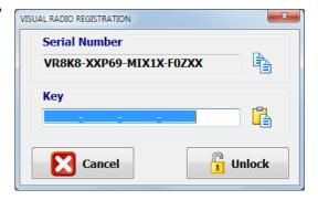
In case your order includes any of those functionalities, the console is supplied from Factory with the functionality activated. If you want to activate it a posteriori, you must copy the "Serial Number" by means of the associated button and send it to AEQ in order to generate the associated "Key" and send it back to you (you must paste it by means of the associated button).
