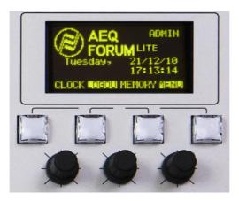
Among the general functions are the instant activation and adjustment of audio effects (EQ, filters, limiters, etc.), configurations and memories management, disconnection of applied effects, phase change, inserting of a test signal, as well as clock, timer and stopwatch for timing control, etc. For more information see chapter "3. DESCRIPTION OF THE INTERNAL MENU" of this manual.
