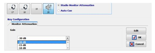
These keys works as follows: when the "Studio Monitor Attenuation" key is not pressed, the studio monitors are muted when a studio microphone is activated.
