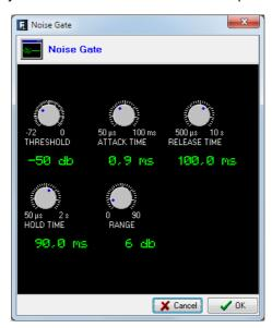
A noise gate is a dynamics processor that lets signals through whose level exceeds a certain threshold, strongly attenuating the signal levels below that threshold and thus muting noise. It enables its user to eliminate extraneous noise from a signal source, whether it is background noise in the studio, in the case of a microphone, or the background noise generated by a playback device, for example, a tape.
