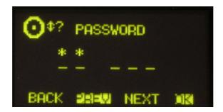
The procedure for entering the password requires the use of the contextual keys beneath the display and any of the three associated encoders.
