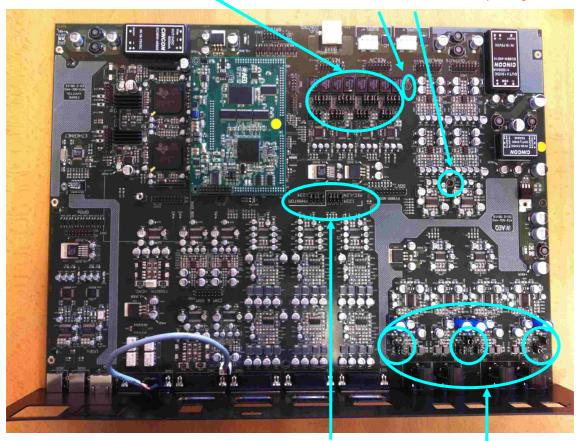
MIC/LINE INPUTS AND PHANTOM POWER PROGRAMMING ZONES
