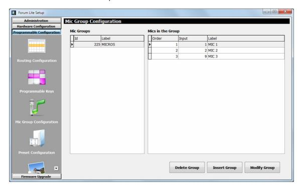
The three buttons at the bottom of the screen allow you to manage the list of groups of microphones and their individual configuration.
