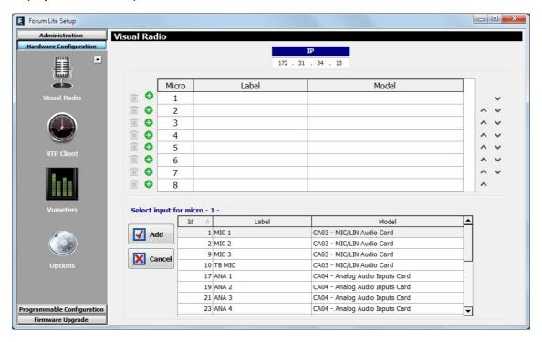
After selecting the desired input and pressing the "Add" button, this input will appear in the list of signals associated with the "Visual Radio" functionality.
