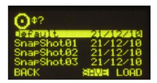
Each stored memory is identified by its name and the date on which it was created. The names of the memories are editable from the configuration software (see section 4.3.5 in this manual).
