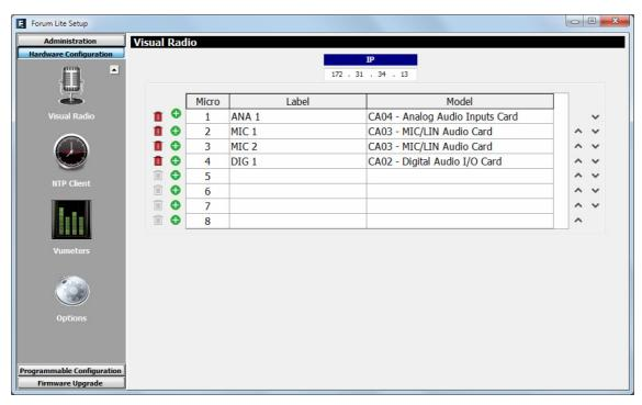
The button **1** allows you to eliminate any of the configured inputs.
