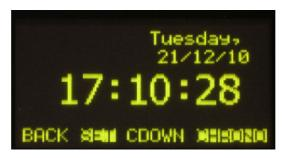
The four options visible on the last line of the display are associated with the four contextual keys below, from left to right:
