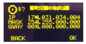
From left to right, the three rotary encoders are associated with "IP", "MASK" and "GWAY" fields respectively. Each one of these fields consist of 4 number separated by dots and named bytes.
