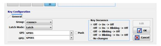
In the case of the **virtual** programmable keys, only the "GPI" that will activate the key and the associated "GPO" should be configured. Besides, the "Push" checkbox must be activated.
