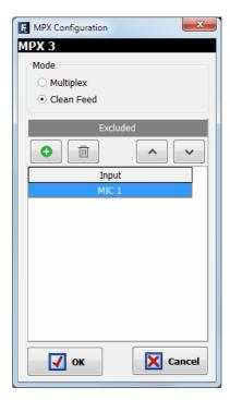
Supposing the configuration of channels activation and routing of the previous image, the "MIC 1" signal defines also in this case an operative **priority 1** for "MPX 3" group because the "PROGRAM" routing key is activated (it doesn't matter that the "AUDITION" and "AUX 2" keys are also activated). This signal will not be sent to "MPX 3" bus because it's excluded from this group.
