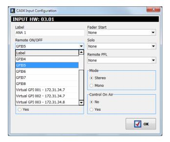
"Solo": allows you to select a physical or virtual GPI (from the list defined in chapter 4.2.1.1) to remotely cut the audio of all the inputs except the one that has been associated with the SOLO function. This is useful when for example multiple microphones are used for the invited guests and the moderator needs to cut all the mics except his own. You can not associate the same GPI to several channels. "None" indicates there is no SOLO function associated with that channel.
