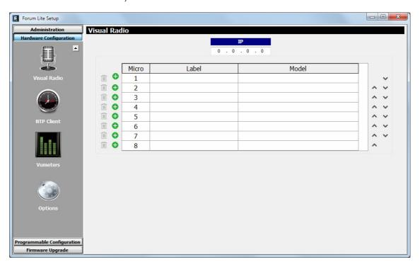
In this submenu first you must configure the destination IP address (it must be in the same subnet of the IP address associated with "LAN" Ethernet port) and then select the input or inputs of the unit (up to a maximum of 8) whose vumeters will be sent to that IP address.
