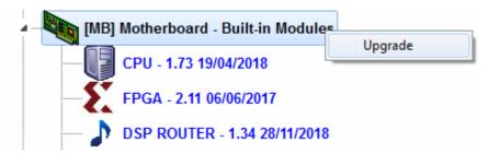
2. In the new window that appears, press the button and select the "AFU" upgrading file (AEQ Firmware Upgrade) that contains the new version you want to load.
