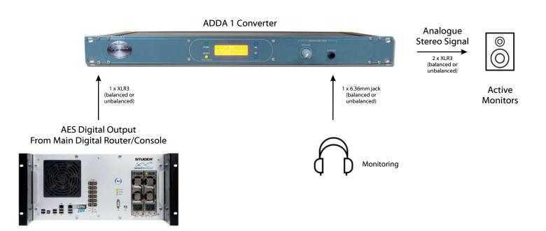
If a broadcast facility largely contains digital connections and you need to connect monitors to a studio, you will need a suitable analogue output.
