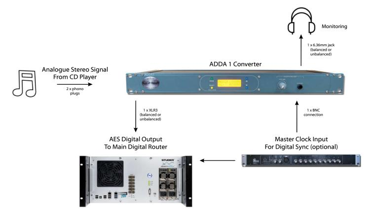
A radio station may be largely digitally linked, with all router and mixer connections via AES. If there are no analogue inputs on the system then the Signature ADDA1 can be used to link the CD player into the digital console.
