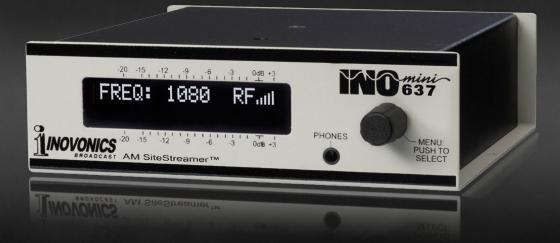
The INOmini 637 SiteStreamer<sup>™</sup> is a Web-enabled medium-wave AM broadcast receiver for remote signal monitoring. Installed at a broadcast transmitter site, or at any remote location with an Internet connection, the unit streams audio from single or multiple (sequenced) off-air sources, or from a hard-wired program audio feed, back to any computer, tablet or mobile device.
