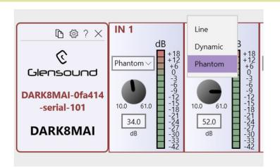
Glen Controller gives full remote control of inputs, gain levels and configuration of any Dark units connected across a network.
