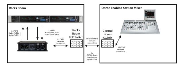
The AoIP22 is the perfect choice for installing in the back of a rack for interfacing legacy analogue audio equipment to your Dante network.
