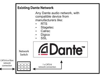
There are over 150 manufacturers that design Dante compatible equipment. In this example, the broadcaster has an established Dante® network. This is most likely to be an audio console, or an intercom system.
