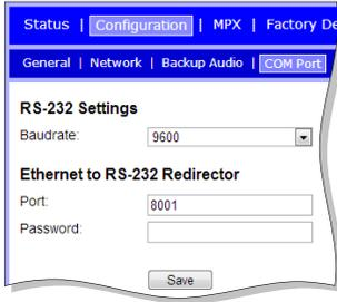
DB9000-STC acts as Ethernet to an RS-232 redirector. You can connect any RS-232 compatible equipment to DB9000-STC and to communicate with it over the Internet. A special software (Virtual COM Port to Ethernet Tool) need to be installed on your PC in order for the COM Port configuration to take place. Enter a Baudrate and configure the external equipment to the same baud rate, specify Port and Password next.
