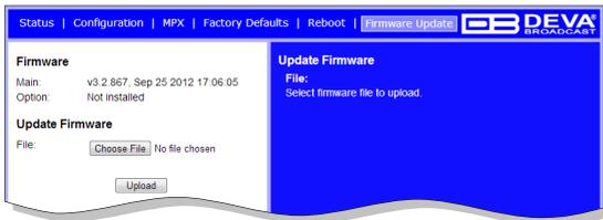
To update the device firmware, please select the new firmware file. Press the Upload button. A dialog window will appear. Confirm firmware update and wait for the process to complete.
