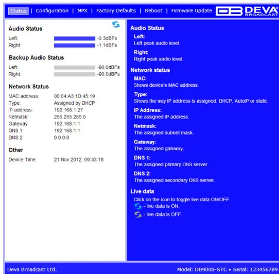
Open a WEB Browser and enter the device IP Address in the browser's address field, then press Enter. The web interface will be displayed Current status information will be displayed comprising: Audio Status; Network Status; Active connections Status.
