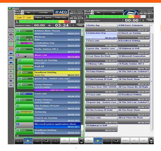
The Broadcast player consists in a set of virtual players for playback/recording, and constitutes the support of the play-out system.
